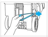
4. Pull belt off of motor shaft.
