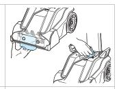
3. Use cloth to wipe clean. Wipe debris from the red filter located beneath where the dirty water tank attaches.
